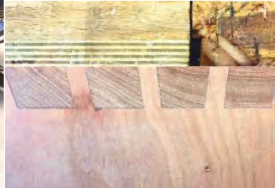
▲ Pic.22 It was then time for some planing using low-angle block and jack planes to achieve a smooth finish, as you can see here
